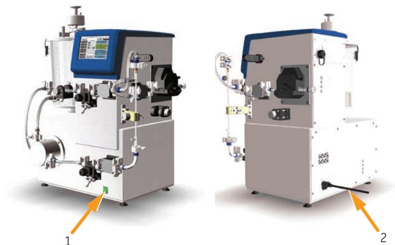
Switch off the mains power supply by pushing the power switch to the 0 position (1), or disconnecting the power cord (2).
