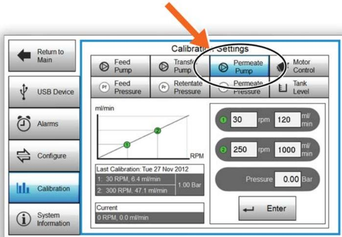
10        Enter the low RPM value of the permeate pump and the corresponding calculated flow value in the gray field indicated with **i**. Assuming that the density is 1, the measured value in g/min will correspond to ml/min.
