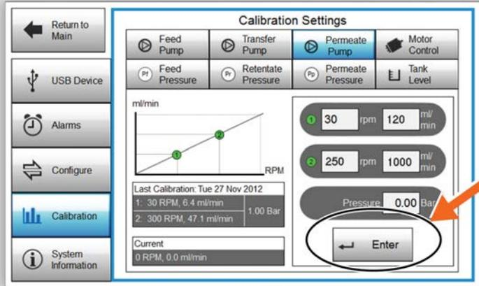
14    To see the flow in ml/min on the main screen after calibration, set the flow rate for the permeate pump to ml/min, see [Set units, on page 167](#).
