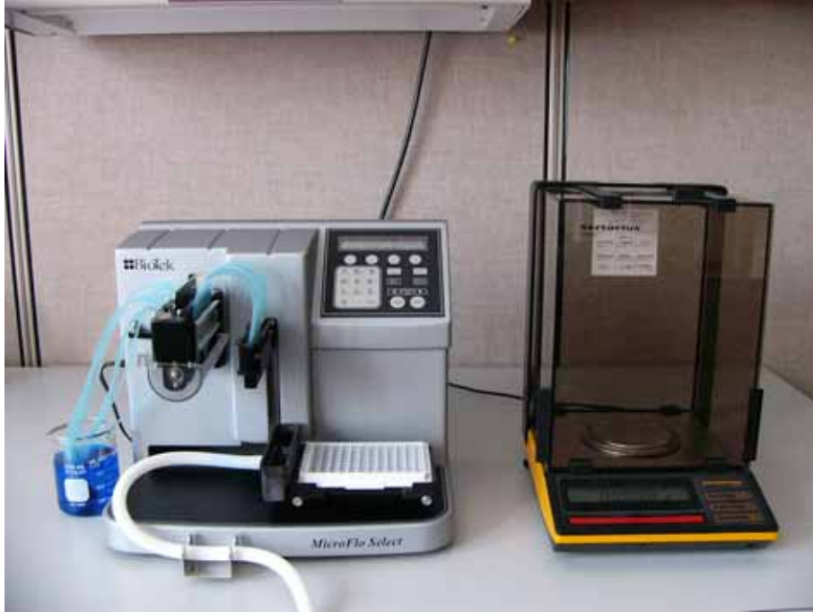
Figure 1: A MicroFlo Select in preparation for the gravimetric cassette calibration, and a digital precision balance with 0.0001 g resolution.
