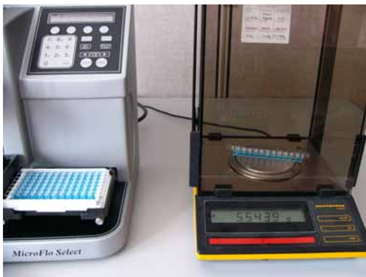
Figure 3: Measure and record the weight of each of the strips after dispensing.
