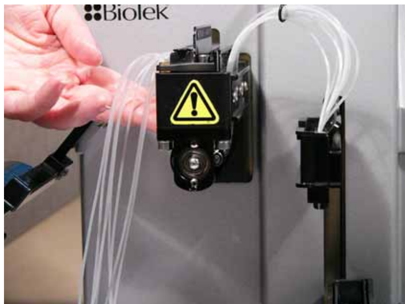
Figure 8: Guide the Tube Tensioner and steel plate into position.
