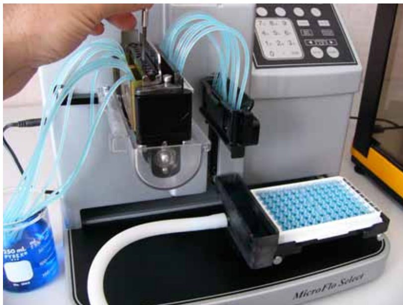
Figure 4: Use the screwdriver shipped with the MicroFlo to adjust the tension in the tubing.
