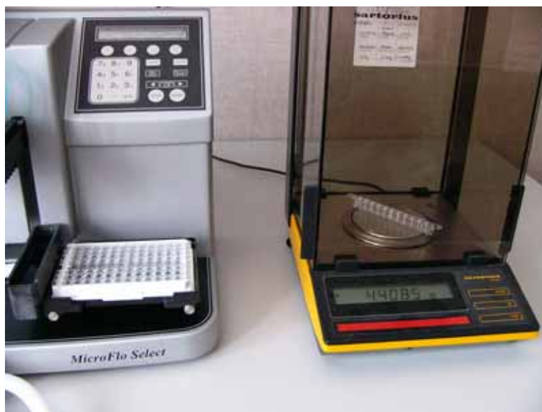
Figure 2: Measure and record the weight of each of the strips prior to dispensing.
